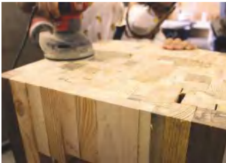
▲ Pic.6 Use a hand-held sander to make the table top smooth, working through the grits up to 220
